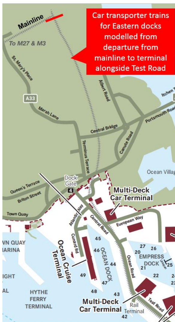
Figure 19 Location of terminal in Eastern docks. Emissions estimated from departure from mainline, shown by red line
